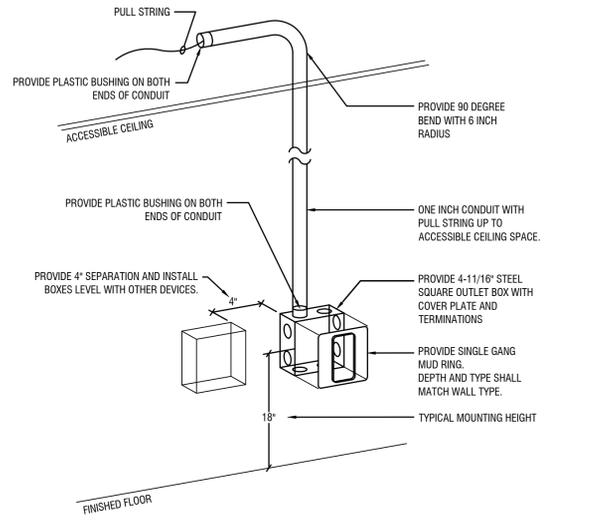
**4 TYPICAL TELE/DATA BOX INSTALLATION DETAIL**
