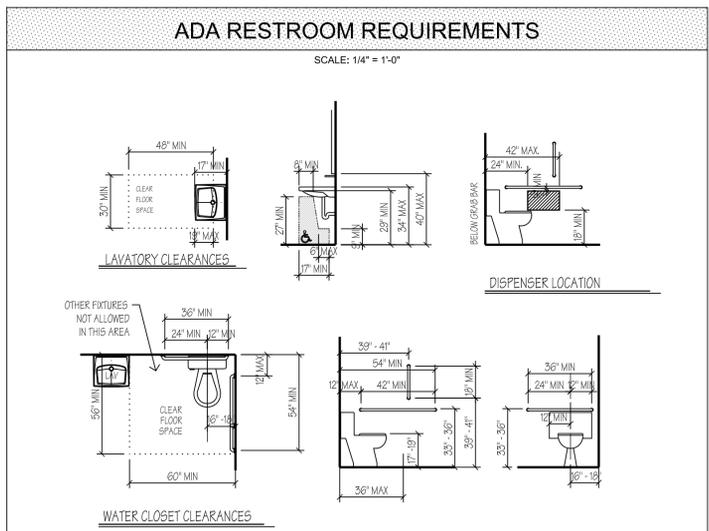
NOTE: WATER CLOSET FLUSH CONTROLS ON OPEN SIDE PER CODE REQUIREMENTS.
